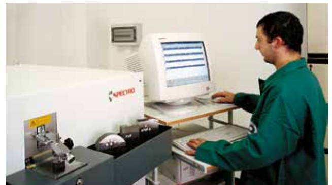
Steel alloy chemistry check
