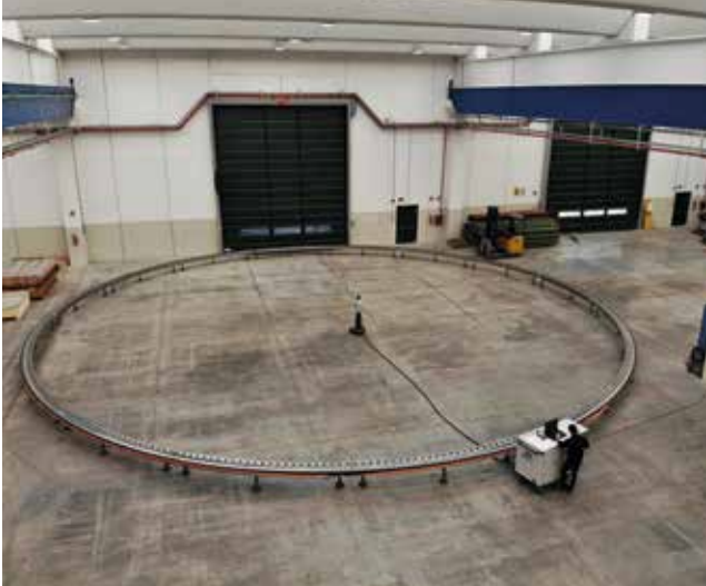
Segmented gear ring
