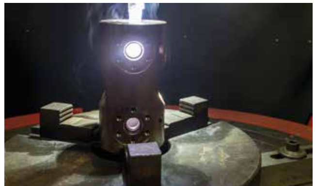
Small internal diameter welding overlays
