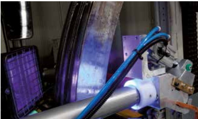
Magnetic particle crack check
