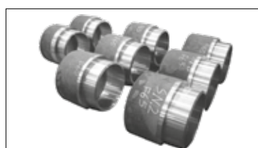
Semi Finished Forged Ring
