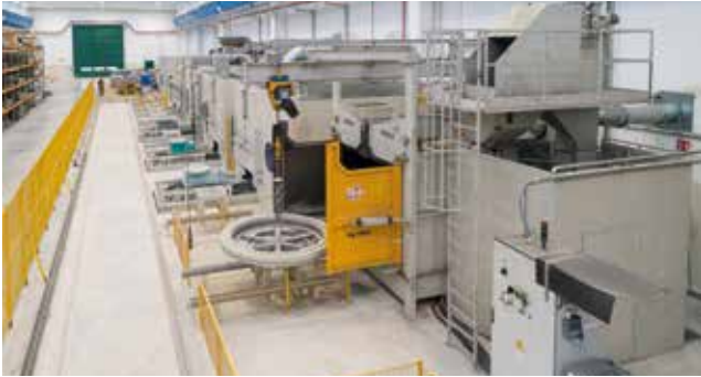
Zinc coating and paint automatic transfer machine
