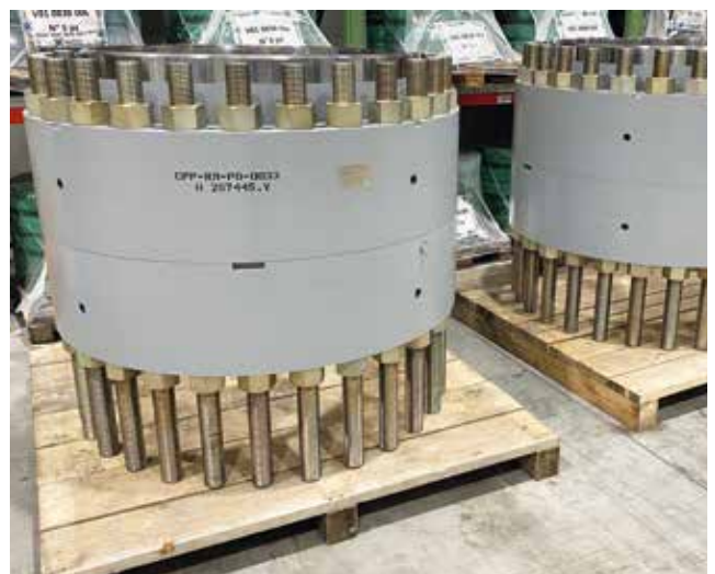
Ball Flange 42" -600 26,8WT F65 + INC625 FULL OVERLAY
