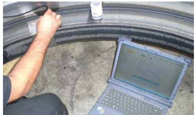
Ultrasonic induction hardening depth verification
