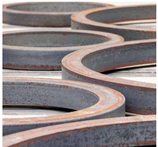
Forged rings ready for machining
