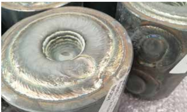
Welded overlays on chamfer/bewel
