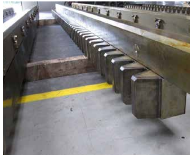
Linear rack single side tooth
