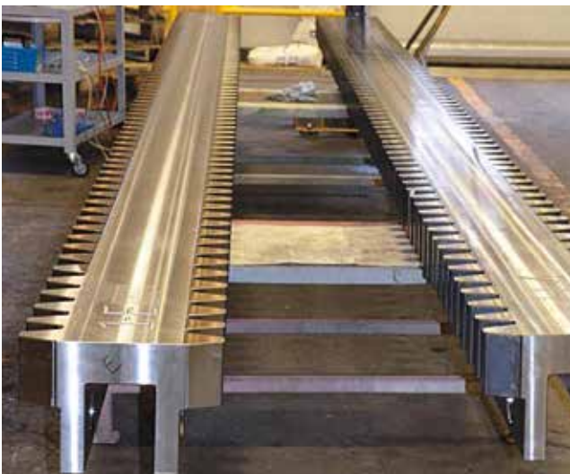
Linear rack dual side tooth
